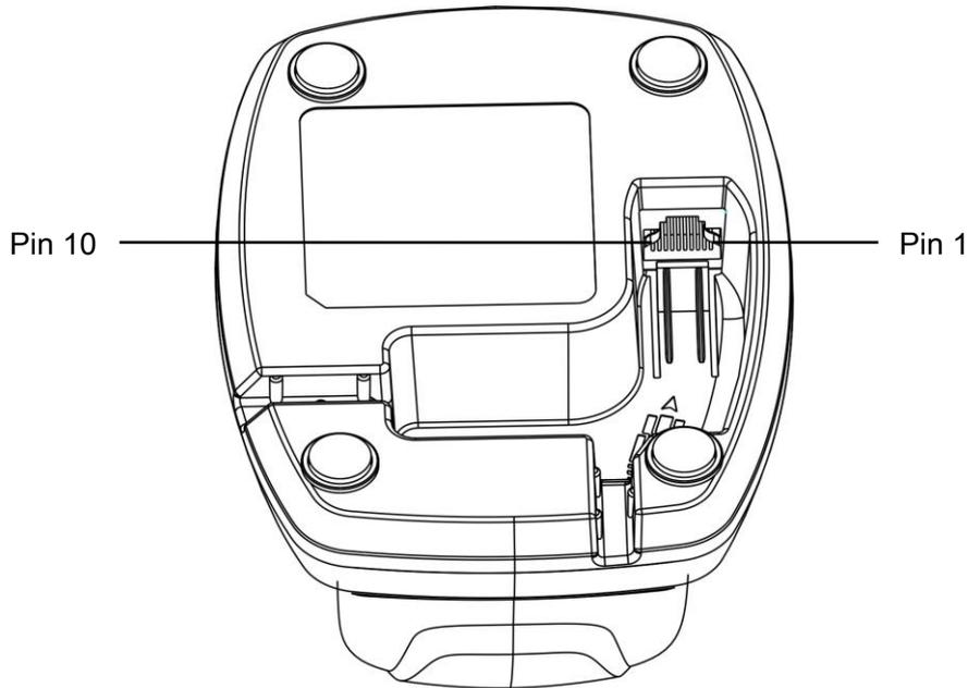
**Figure 2-1 Cable connector interface pin-outs**
