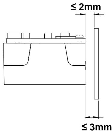
If the window is required to be in a tilted position, the above distance requirements should be met and tilt angle should ensure no reflections back into the lens.
